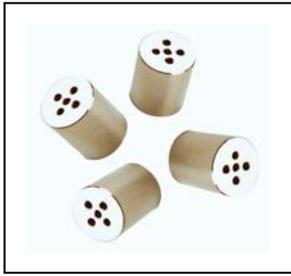
The MP418 is a 1/4" free-field prepolarized microphone. It was developed based on BSWA's Type 1 microphone technologies. MP418's frequency response meets IEC61672 Class 2 requirements. Each microphone is individually calibrated and aged at 80°C for long-term stability and reliability.
