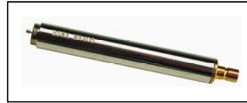
The MA408 is 1/4" preamplifier using SMB connector for the output while the threads for the microphone comply with the IEC61094-4 WSF3 standard. This makes it suitable for use with any standard prepolarized 1/4" microphone.
