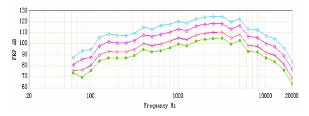
Frequency Response of VSS210 Measured at 5 cm from Outlet in the Anechoic Chamber
