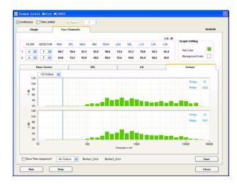
VA-Lab ENV is a powerful sound level meter. It supports 10 channel sound pressure level measurements at 10 locations. Each channel can perform multi-task analysis such as statistical levels, 1/3 octave, and levels vs. time.
