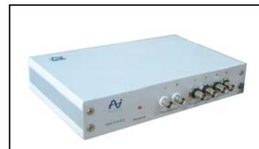
The MC3242 is a 4-channel hardware designed using NI 9233 data acquisition card. It can analyze acoustic and vibration signals acquired simultaneously from its 4 channels. MC3242 has two signal output channels.
