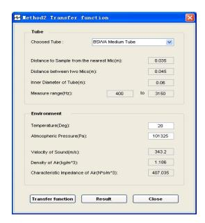
The Transfer Function Method uses two fixed microphones to acquire sound pressure near the sample. VA-Lab IMP can accurately separate the incident wave and reflect wave, then calculate the absorption coefficients. An extended frequency range can be obtained from the combination of measurement results gained in different diameters of the tubes. It automatically calculates the acoustic properties of material at a wide frequency range of interests.
