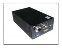
The VSS210 Volume Source is a mid-frequency volume source. It is ideal acoustical source for reciprocity measurements and TPA analysis. VSS210 uses a power speaker driver to deliver up to 125 dB over the frequency range from 200 to 10,000 Hz.
