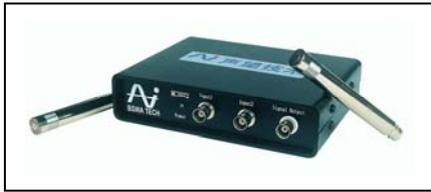
The MC3022 is a USB powered Plug-N-Play measurement soundcard with two ICP input channels and one output source channel. MC3022 is based on 16 bit A/D converters with two-channel simultaneous sampling frequency of 44.1 kHz. It is the perfect start to building your own two-channel sound and vibration measurement system.
