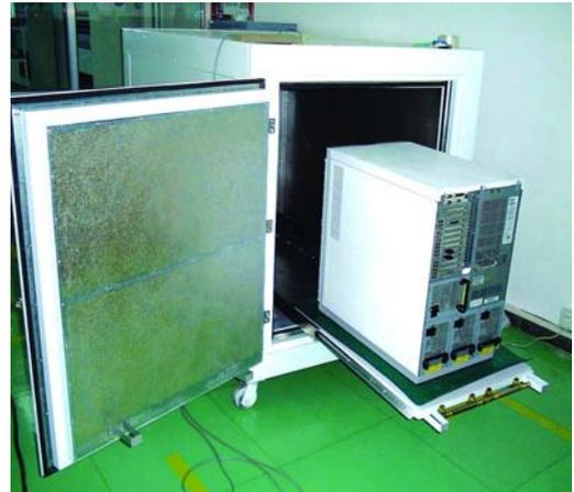
The XS Series Anechoic Test Box is made from steel sandwich panels with sound absorption material as fillings. The internal surface is perforated to provide sound absorption, while the external metal panel provides the sound insulation. Optional Sonex sound absorption foam can be added to the internal surface to increase the total absorption.
