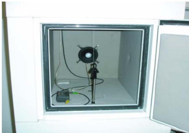
The Anechoic Text Box is a low cost alternative to the anechoic chamber. The correction factors can be determined by comparison of the measurements in the chamber and box.
