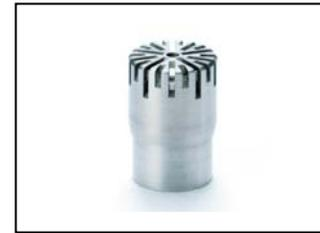
The MK401 is 1/4" free-field microphone required a polarization voltage of 200 V. The frequency range of MK401 is from 20 Hz to 70 kHz and meets IEC 61672 Class 1 requirements. The dynamic range of MK401 is up to 170 dB, which makes MK401 the best choice for high intensity and top loudspeaker testing.
